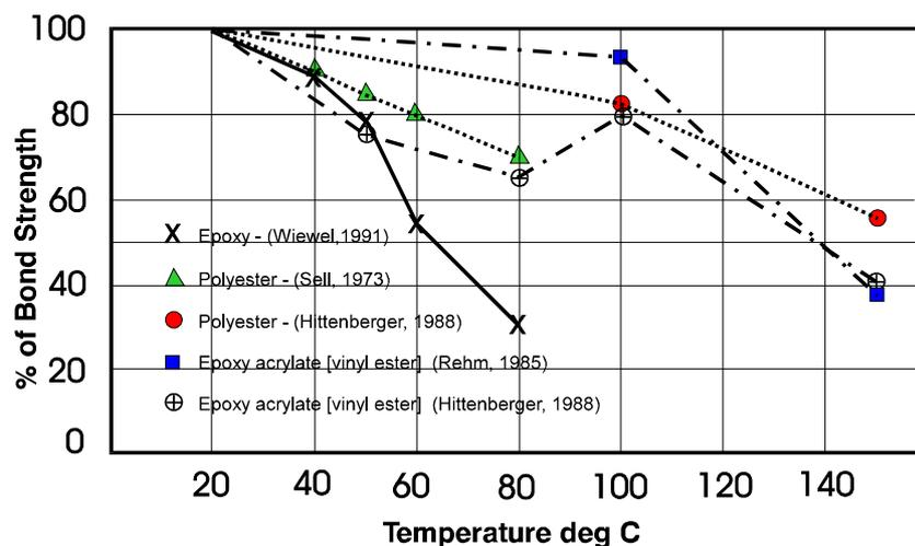
Figure 6 Effect of heat on chemical anchors (8)
