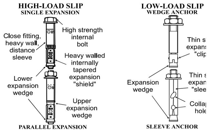
**Figure 9 Load controlled expansion anchors**
