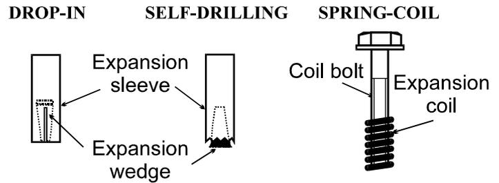
Figure 10 Deformation controlled expansion anchors
