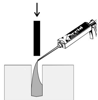
Figure 12 Injection chemical anchor
