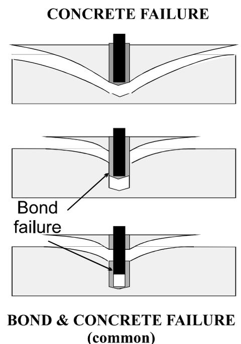
Figure 1. Grouted & chemical anchors
