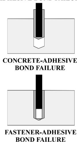
Figure 5 Bond failures
