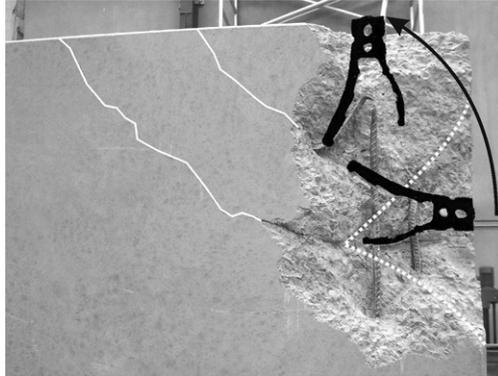
This photo of the failure shows the initial (horizontal) position of the anchor and its final position superimposed over the failed surface. The initial shear crack is identified by a broken white line and the final shear cracks extending from the hanger bar have been mapped with firm white lines.
